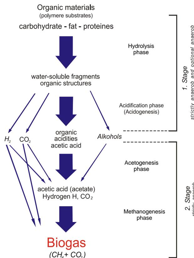
Figure 2 – The anaerobic degradation phases
