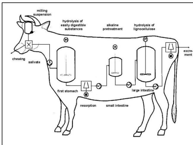
Figure 1 - Hydrolysis analog to ruminant digestive
